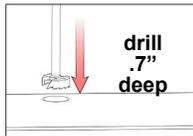
3. Drill a 1/2" diameter hole in the center of the hole that was drilled in Step 2. Drill completely through the deck board with this bit.
