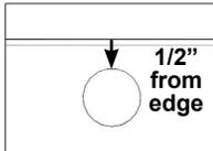
2. Use a 1" Diameter Forstner Bit to bore a flat bottom hole .7" deep into the deck board.
