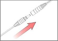
7. Connection is fully engaged when there is minimal gap between the male and female connector.
