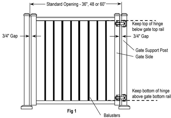
2. Follow installation instructions included with hinges and latches. **NOTE:** Align gate rails with adjacent railing when attaching gate to gate support post.
