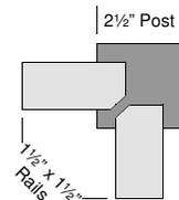
**Cutting Down Sections:** To cut down a section, determine the length of section needed. Mark and cut. Notch end of rails using the Regis Notching Tool and install as above.
